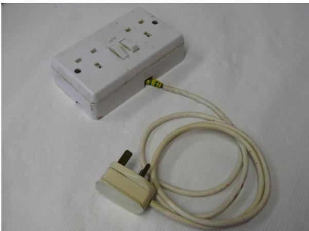
A closer look highlights that the extension lead was made without an earth cable! (Using a 2-core
