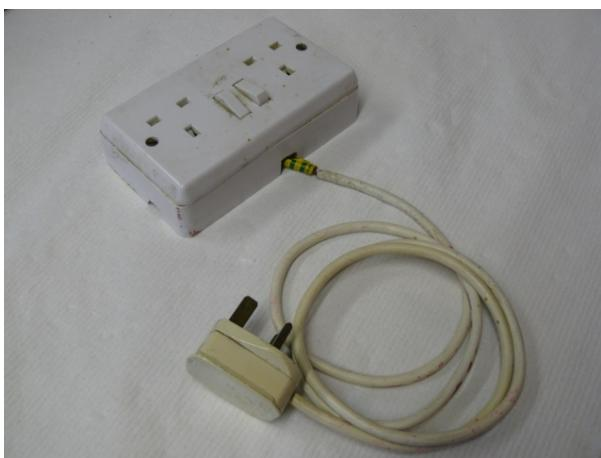
A closer look highlights that the extension lead was made without an earth cable! (Using a 2-core cable, brown and blue only). The earth cable is needed to protect you from an electric shock in the event of a fault developing within the appliance. Please do not use homemade leads or appliances.
