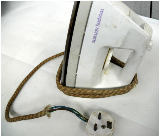
Many of us will have attempted to 'repair' a cable with tape. Tape is not a permanent repair and appliances in this state should not be used. Unfortunately most cables on appliances such as irons cannot be replaced and the appliance has to be replaced.
